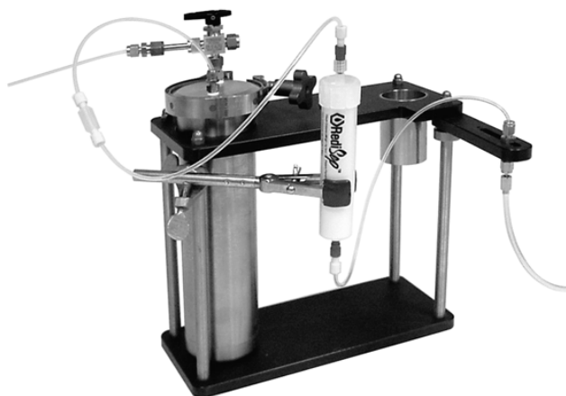
Figure 1: RediSep column on pressurized solvent reservoir system
