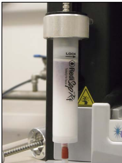
Figure 1: 25 g self-pack column installed on a CombiFlash Rf system
