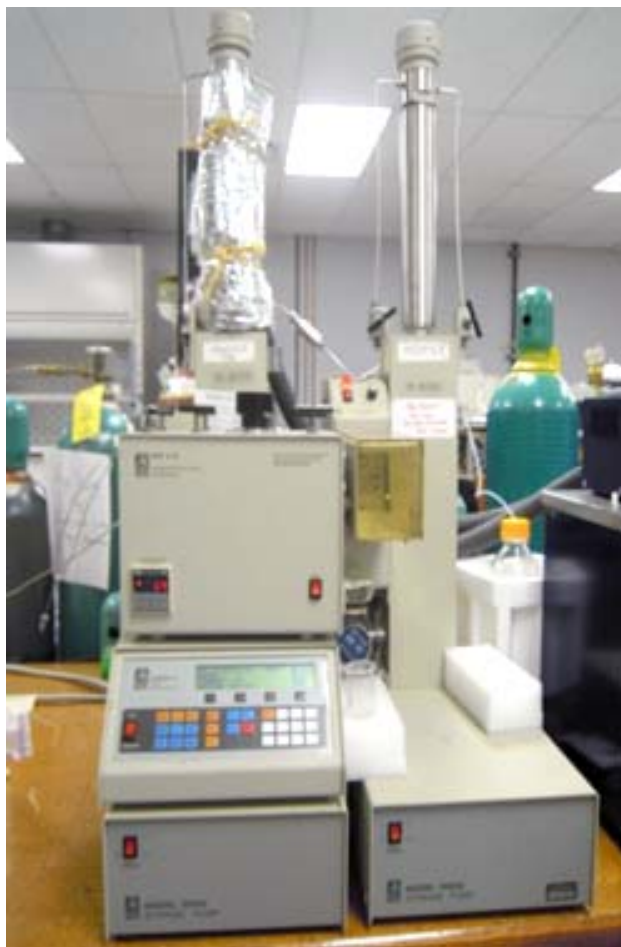
Figure 1: Photo and Schematic of the Supercritical Fluid Cleaning of Archaeological Artifacts
