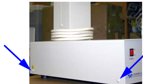
Figure 4: Pump case top screws (2 of 4 shown)
