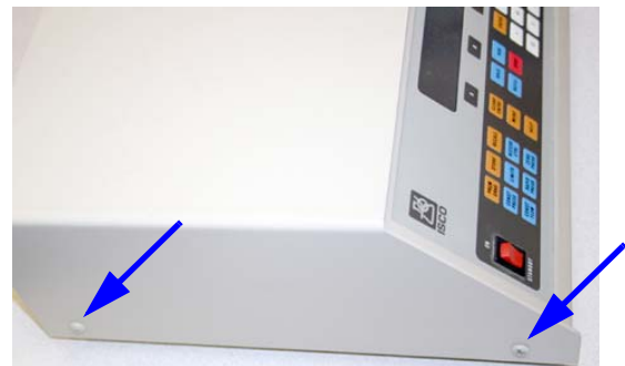
Figure 3: Controller case top screws (2 of 4 shown)
