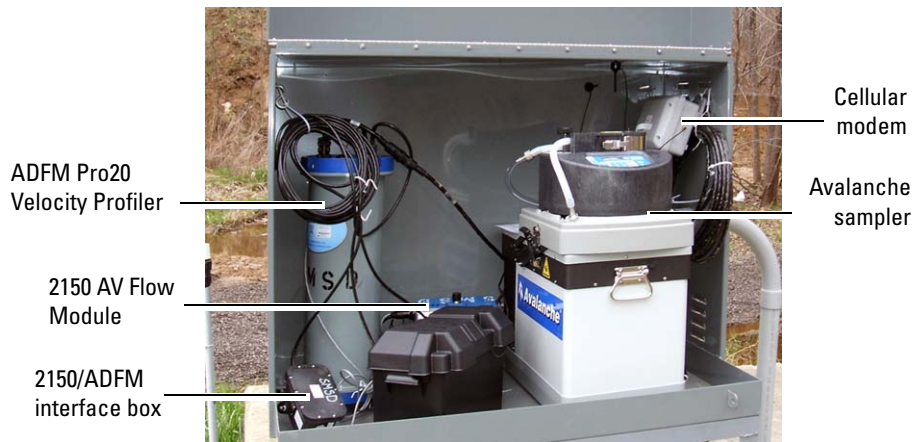
Figure 3: Avalanche sampler in environmental enclosure With cellular modem, ADFM Pro20 Velocity Profiler, and 2150 Area Velocity Module
