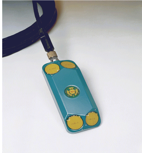
Figure 3. ADFM transducer assembly. Opposing beam pairs are situated on either side of the transducer (on the long axis). The depth detecting vertical transducer ceramic is in the middle of the assembly.
