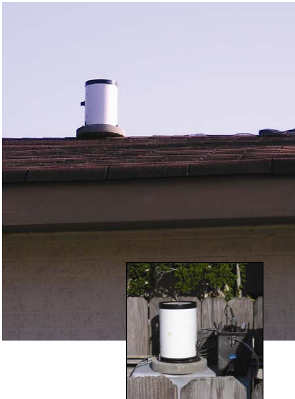
The separate rain gauge and logger allow great flexibility in setting up for a wide range of monitoring site requirements.
